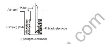
A platinum wire is welded to the Pt strip and sealed in a glass tube as to make contact with outer circuit through mercury. The Pt strip is placed in an acid solution which has H<sup>+</sup> ion concentration 1 M. Pure H<sub>2</sub> gas circulated at 1 atm,  $H_2 = 2H^+ + 2e^-$ .
